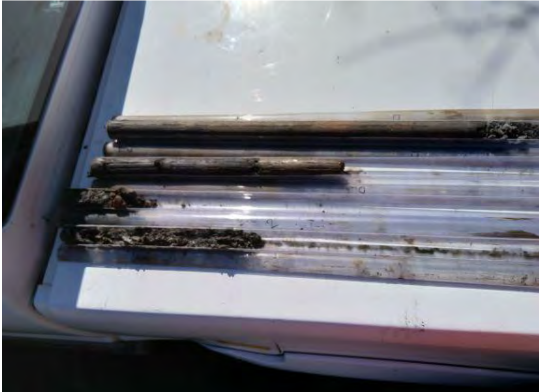
Photo 7: BH106 push tube sample showing loss of sample return
