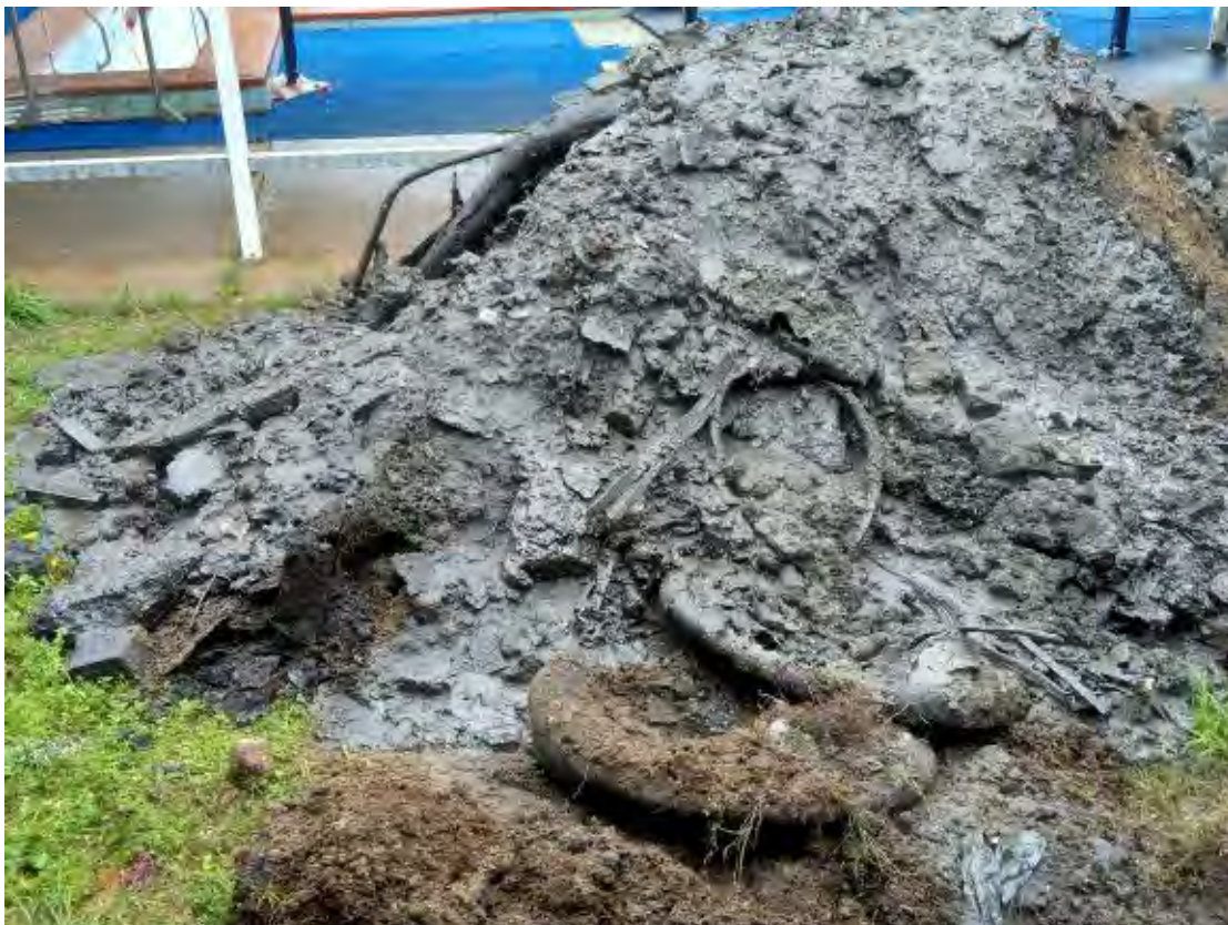
Photo 2: TP121 looking east showing fill material from beneath water table
