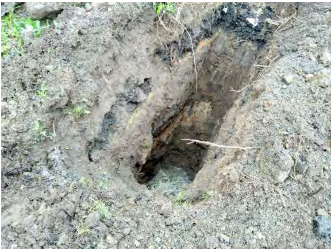
Photo 8: TP124 looking east showing soil profile with groundwater seepage at base of excavation
