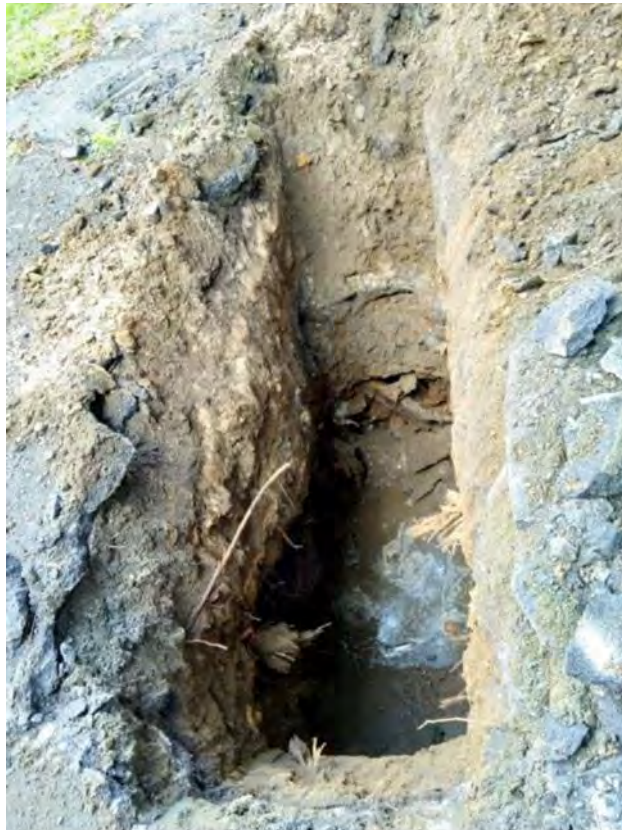
Photo 6: P128 looking east showing soil profile and groundwater at base of test pit
